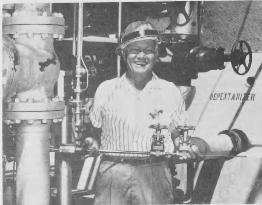
A PROBE-type sample connection for product lines is positioned by J. C. Walker, assistant shift foreman in Process-Cracking and Light Ends. Its use was suggested by Mr. Walker who was awarded a Fls. 700 CYI award in August. His idea was also named the CYI-of-the-Month.
